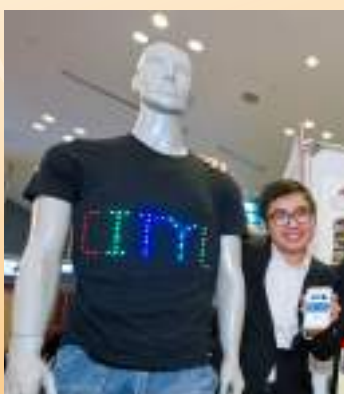
Tamar Wong Hei-ting (Creative Media, Year 4) invented the Wearable Canvas, a wireless LED-fitted T-shirt with a drawing app that allows tailor-made text or design patterns to be instantly displayed on the fabric.
