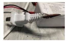
During the investigation, it was also discovered that a 2-pin plug, lacking grounding and a fuse, was in use. This contravenes EMSD regulations. The electrical wires were not properly connected or protected, leading to exposed copper wires.
