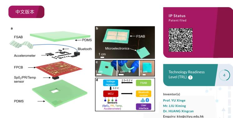
a) Exploded view of the device, represented layer by layer. b) Four sweatactivated batteries on 8cm×8cm flexible substrate connected to the soft microelectronic. (3cm×3cm) c) The flexibility of the soft microelectronic under pressure. d) The diagram of the device's working principle.
