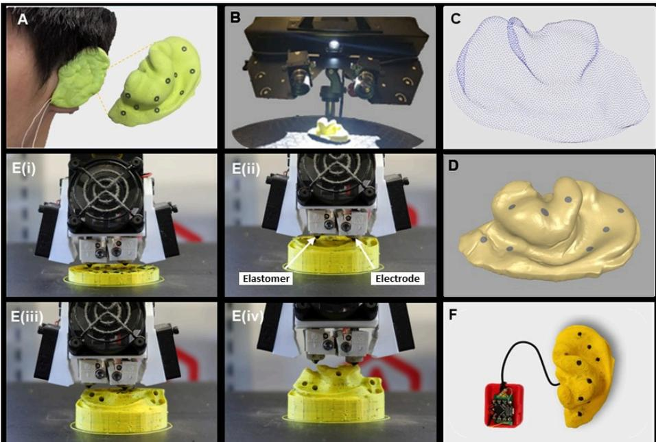
Fabrication process of 3D-PAS. (A) Human-specific auricular impression molding. (B) 3D-scanning of reverse auricular mold. (C) Points cloud generating. (D) Geometric designing and locating of embedded electrodes pathways. (E) 3D-printing of sensor with elastomer and functional material. (F) Prototype of
