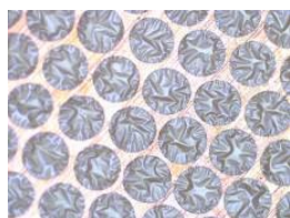
Fig. 2 Si Film supported by 300-mesh copper grid (without carbon film).
