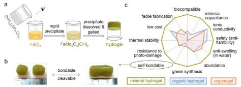
Schematic illustration of the synthetic route of the mineral gels reported in this study (a), the optical photographs of two pieces of the mineral gel before and after merged into one (b), and their general characteristics in comparison with organic hydrogels and organogels (c).
