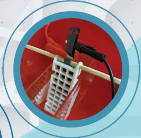
A functional prototype built with the first design of an innovatively designed sleeve that holds their electrode mesh panels at a precise distance between the anode and cathode.
