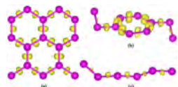
Fig. 4 ELF isosurfaces of (a) Cmcm - \text{Mn}_2\text{B}_3 , (b) C2/m - \text{Mn}_2\text{B}_3 and (c) C2/c - \text{Mn}_2\text{B}_3 . The ELF isosurface value is 0.5.
