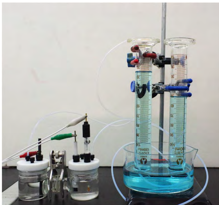
Figure S11. Photograph of the water splitting system with the MoON-2 electrocatalyst and O 2 (left) and H 2 (right) gas generation determined by the water displacement method.
