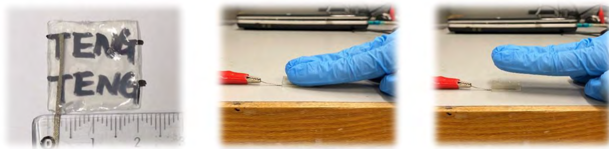
Figure S8. Photographs of the AV/LiCl organohydrogel-based TENG and its contact and separation with nitrile glove for output measurement.
