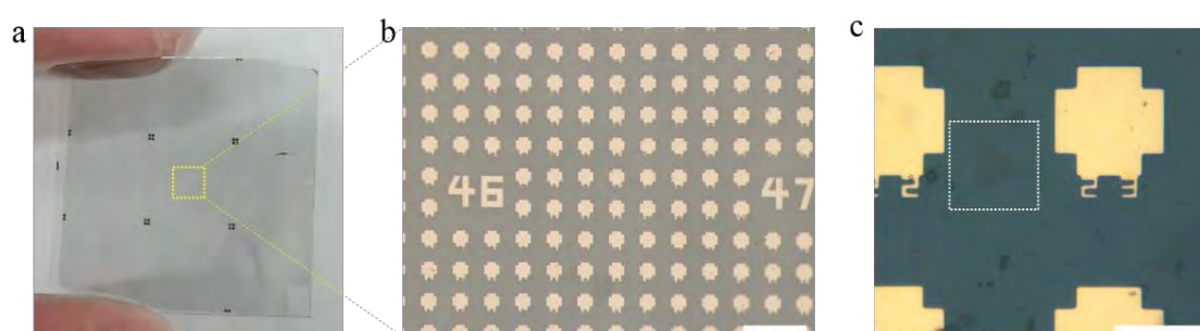
Figure S21. Optical images: (a) Marked PET substrate, (b) Magnified image of the dashed yellow area in (a) (Scale bar: 200\ \mu\text{m} ), and (c) Transferred monolayer \text{Mo}_{0.46}\text{W}_{0.54}\text{S}_2 alloy on PET substrate (Scale bar: 40\ \mu\text{m} ).
