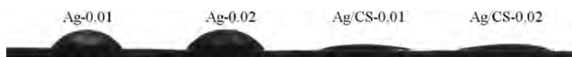
Figure 4. Images of water droplets lying on flat Ag doped and Ag/CS capped TNWs.
