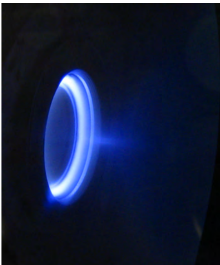
FIG. 6. Photograph of the discharge in the enlarged cylindrical-anode-layer Hall plasma accelerator.
