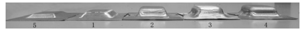
FIG. 11. Cups drawn using different electric current parameters: sample 4 with optimal electric current parameters: punch speed = 7.5 mm/min, punch stroke = 12.5 mm; sample 5 with no electropulsing: punch speed = 5 mm/min, punch stroke = 3.5 mm.
