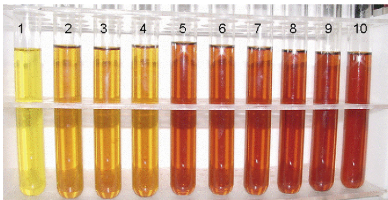
Fig. 42. Enzymatic activity test of original and ion beam mutated xylanase producing strains. (1) Control tube without bacteria; (2–4) original strain showing basic levels of xylanase activity; (5–10) mutated strains showing increased enzymatic activity.
