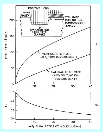
The etching rate can be enhanced by ion-assisted chemical reactions.
