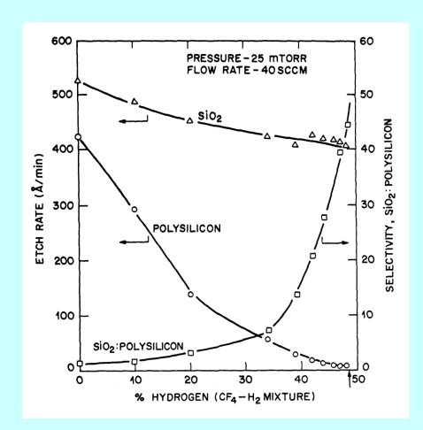
When a gas is mixed with one or more additive gases, both the etch rate and selectivity can be altered.
