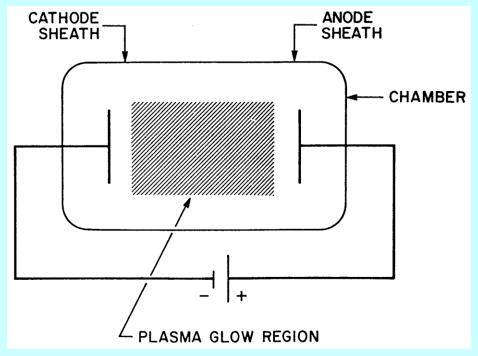
A plasma is produced when an electric field is applied across two electrodes between which a gas is confined at low pressure, causing the gas to break down and become ionized.
