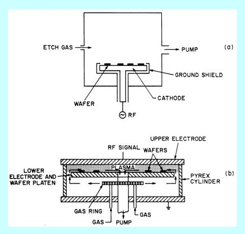
(**Top**) Sputtering - etching system: Inert gas ions accelerated by the applied electric field sputter off the surface. There is essentially no sputtering of the sidewalls to attain a high degree of anisotropy, but the selectivity is poor.
