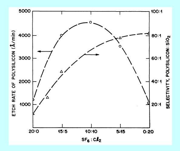
The etching rate of silicon can be adjusted to be 10 to 80 times faster than that of silicon dioxide by varying the gas composition of sulfur hexafluoride ( $SF_6$ ) and chlorine.
