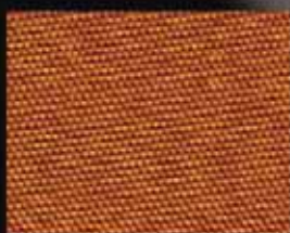
Contact mode atomic mica lattice at 0.6Hz
